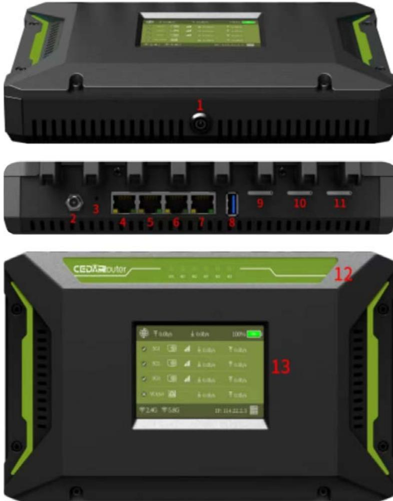
1. ON/OFF: The power on/off button of the bonding router.
